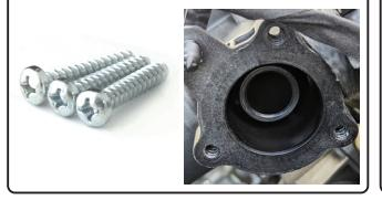
Where the diverter valve mount has metal threaded inserts as shown below, use the supplied fine-pitch screws (requires a 5mm hex key). Tighten to 6-8Nm (4.4-6lbf-ft).
