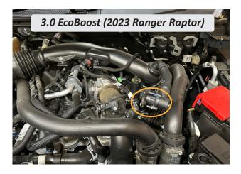
1) Remove the electrical connector from the factory diverter valve. First slide the grey locking tab out, then push it down to unclip the connector:
