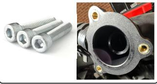
6. Position the VTA onto the car. NOTE: The bolt pattern is NOT symmetrical, so you will need to ensure the body is oriented correctly so all three screw holes line up. Don't worry about the orientation of the connector, as it can be rotated by hand to a position that best suits your application.
