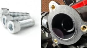
6. Position the DV+ onto the car. NOTE: The bolt pattern is NOT symmetrical, so you will need to ensure the body is oriented correctly so all three screw holes line up. Don't worry about the orientation of the connector, as it can be rotated by hand to a position that best suits your application.
