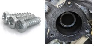
Where the diverter valve mount has metal threaded inserts as shown below, use the supplied fine-pitch screws (requires a 5mm hex key). Tighten to 6-8Nm (4.4-6lbf-ft).
