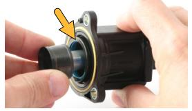
Pull the piston and spring out of the body, then remove the yellow o-ring. This will leave the plastic ring indicated by the arrow, which MUST BE REMOVED before the DV+ is installed. Lever it gently and work your way around.
