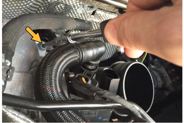
Rotate the top of the intake elbow towards the firewall to disengage it from the turbo.
