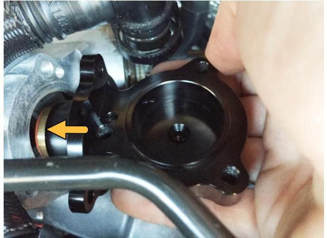
Insert the GFB plunger spring into the diverter solenoid, followed by the plunger. Put the yellow factory o-ring on top of the DV+ body. Hold the plunger with your finger and fit the solenoid assembly onto the DV+ body.
