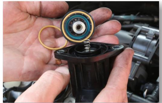
4. Assemble the GFB parts onto the factory solenoid coil as shown in the exploded view below, making sure to use the GFB-supplied plunger spring, and the two yellow factory o-rings.
