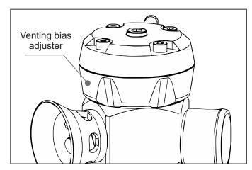
Turning the Respons venting bias adjuster fully clockwise completely opens the trumpet port and gives the loudest sound, whilst setting it fully anti-clockwise results in 100% recirculation venting, which is the same as the stock valves and is the quietest operation. You can set the adjustment anywhere in between for a variable venting ratio and to control the sound volume.
