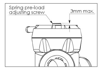
setting is achieved when the top of the adjustment screw is 3mm above the head of the valve as shown opposite. Do not set the screw more than 3mm above the head.
