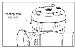
provided the spring pre-load is correctly set. However, some engine modifications can make the car more sensitive to atmosphere venting, which can lead to backfiring or idle issues if the valve isn't adjusted accordingly. If such issues cannot be corrected with the spring pre-load alone, they can be cured by reducing the atmosphere venting bias until the problem is resolved – this is one of the key benefits of GFB's venting bias adjustment feature.
