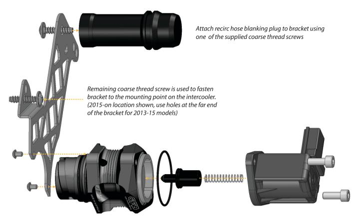
Screw bracket to VTA body using supplied M4x6 screws. Loctite or similar threadlocker is recommended
