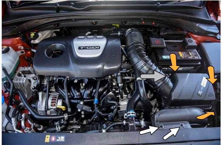
2) Before unbolting the factory valve, it is easiest to first remove the recirc hose while the valve is still solidly mounted (this hose is quite tight and needs some wiggling persuasion). Then remove the factory valve from the car using a 10mm socket for the 4 screws.
