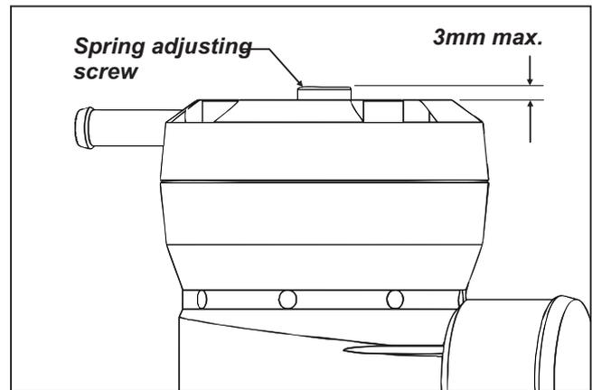
Since the Mach 2 valves are fully recirculated, and there is no MAF sensor on these cars, the spring pre-load adjustment is not critical and is it possible to use the Mach 2 valves straight out of the box without adjustment. However, you can use the adjustment to fine-tune throttle response. Generally speaking, the hardest spring pre-load you can run without causing compressor surge (fluttering sound when lifting off the throttle) is ideal.
