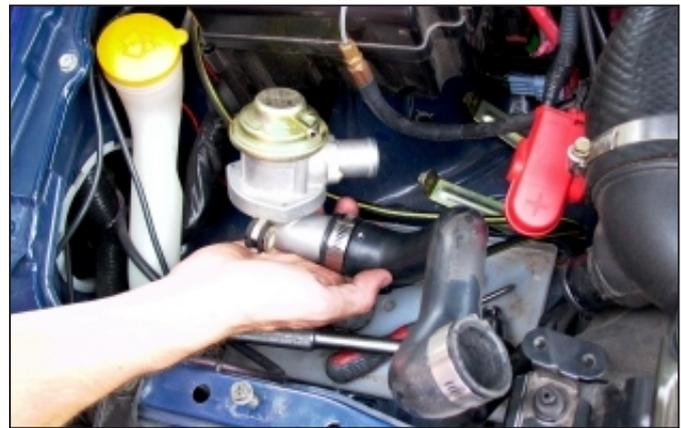
5) Remove the factory valve from the lower elbow by undoing the 3 screws on the underside of the flange.
