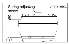
It is therefore possible to use the Mach 2 straight out of the box without any spring pre-load adjustments, however you can use the adjustment to fine-tune throttle response. Generally speaking, the hardest spring pre-load you can run without causing compressor surge (fluttering sound when lifting off the throttle) is ideal.
